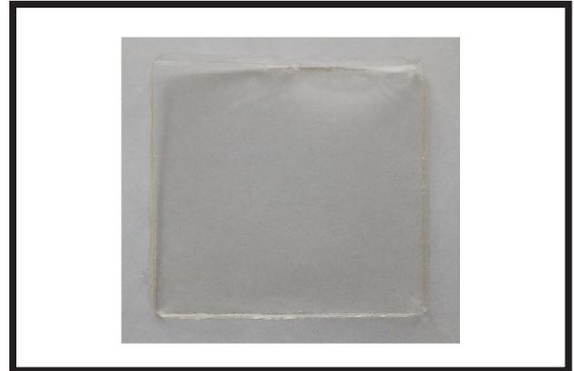
FIG. 1. An example of a film made from fish collagen.
